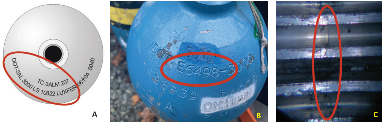
Figures A-4: A) DOT marking on aluminum alloy 6061-T6 cylinder, Credit Luxfer; B) DOT marking on aluminum alloy 6351-T6 cylinder, correctly recertified. Credit M. Gresham; C) Sustained load crack on cylinder internal thread. Credit F. Burman
