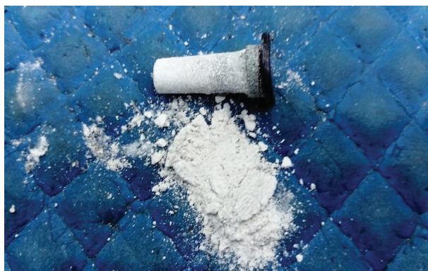
Figure A-3: Regulator inlet filter clogged with aluminum oxide. Credit: J. Polanco
