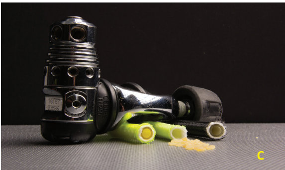
Figures A-2: braided hose failure: A) Inflator hose clearly kinked. Credit DAN, B) Branded breathing hose intact; unbranded inflator hose clearly degraded. Credit DAN; C) Regulator low pressure chamber filled with debris. Credit DAN; D) Second stage inlet clogged with hose debris. Credit DAN.
