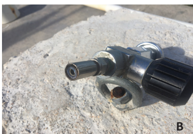
Pictures A-1: A) Filling whip burst at the manifold valve. Credit S. Prosterman; B) Clear indication of failure at the crimped fitting. Credit S. Prosterman. C) Typical whip restraint. Credit Chicago Coupling.
