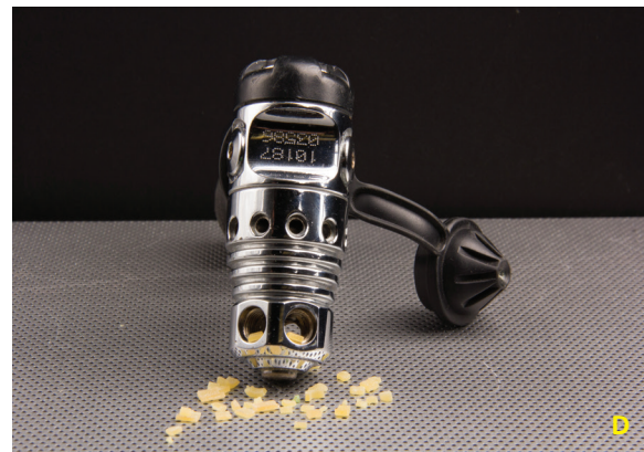
Figures A-2: braided hose failure: A) Inflator hose clearly kinked. Credit DAN, B) Branded breathing hose intact; unbranded inflator hose clearly degraded. Credit DAN; C) Regulator low pressure chamber filled with debris. Credit DAN; D) Second stage inlet clogged with hose debris. Credit DAN.
