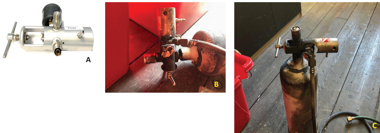
Figures A-5: A) Aluminum version of Allied multifunction regulator. Credit F. Burman B-C) Aluminum multifunction regulator fire damage. Credit DAN Europe.
