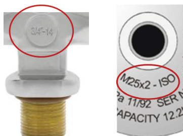
Figures A-7: Different cylinder valve configurations: A) ¾- 14 NPS (National Pipe Straight), United States standard, DGX DX-722401-O2; B) M25 x 2 - ISO, international harmonized standard, IMCA SF 01/16.
