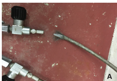
Pictures A-1: A) Filling whip burst at the manifold valve. Credit S. Prosterman; B) Clear indication of failure at the crimped fitting. Credit S. Prosterman. C) Typical whip restraint. Credit Chicago Coupling.
