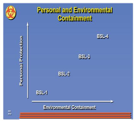
**FIGURE 2.1** Personal protection plotted against environmental containment, showing the distribution of the containment levels along these two metrics. SOURCE: Thomas Ksiazek.
