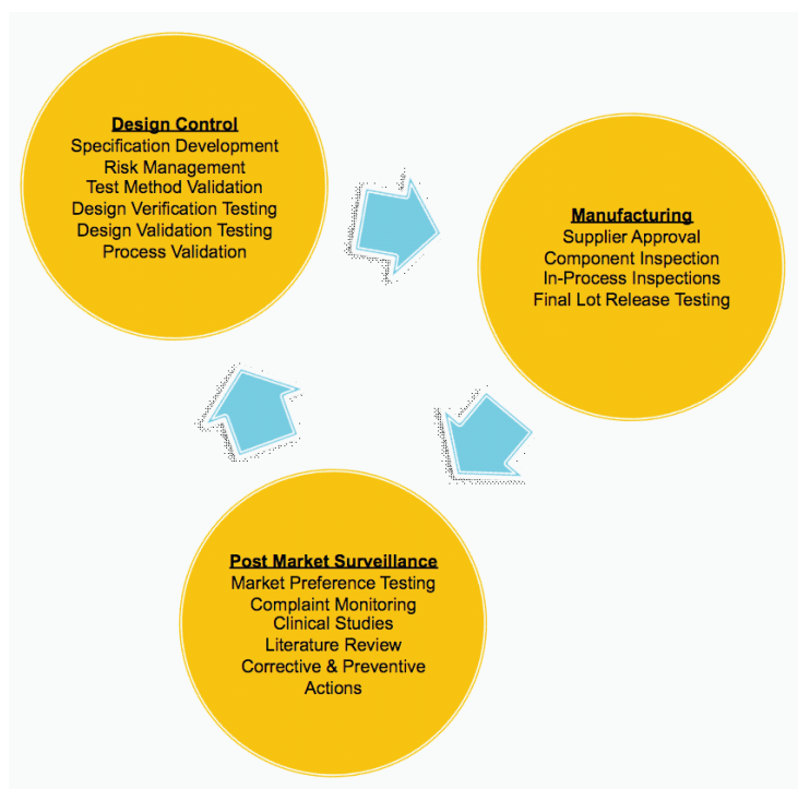
FIGURE 4-1 Patient safety is delivered primarily through good quality systems. Design control designs quality into a product from the beginning of development. Quality systems follow the product through its life cycle into the market.
