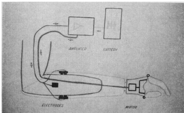
Fig. 1.—Diagram indicating the connections of the apparatus from the battery and amplifier to the motor in the hand. (See text.)
