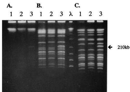
FIG. 3. Strain ATCC 824 contains an extrachromosomal element which is missing in DG1 and M5. Ethidium bromide-stained unrestricted total DNA (A) from M5 (lane 1), DG1 (lane 2), and ATCC 824 (lane 3) or total DNA digested by *Sst*II (B) or *Sma*I (C) after separation by PFGE is shown. Lane  $\lambda$  contains concatemers of lambda DNA *c*1857 *ind*1 *Sam*7 (NEB) used as molecular size standards.
