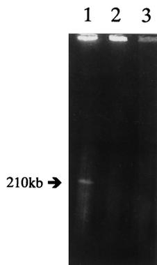
FIG. 4. Strain ATCC 824 contains a circular 210-kb plasmid which is missing in DG1 and M5. Total DNA plugs were digested by *Eag*I, linear fragments were then removed from the plugs by PFGE and treated with *Sst*II, and residual DNA fragments from ATCC 824 (lane 1), DG1 (lane 2), and M5 (lane 3) were separated by PFGE and stained by ethidium bromide.
